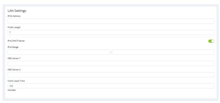
IPv6 Address: Enter the LAN IPv6 Address.
