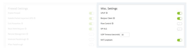
**UPnP:** This enables Universal Plug and Play, a protocol that permits the network to discover and operate devices and applications seamlessly.
