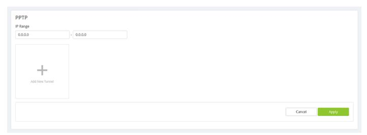
Click the + Add New Tunnel button to create a new PPTP tunnel. Enter the tunnel name, and a username and password for that user.
