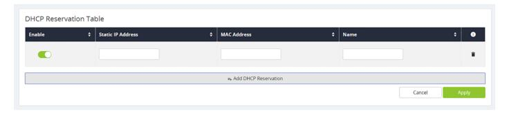
Click the Add DHCP Reservation button to add a device. The IP address must be in IPv4 format.
