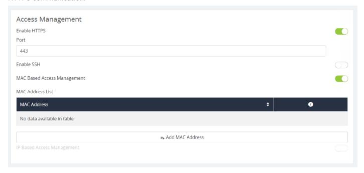
Enabling SSH enables encryption for the secure use of the Command Line Interface on port 22.
