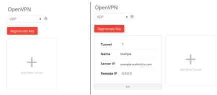
There is a toggle for **UDP** or **TCP** protocol, when configuring an OpenVPN Tunnel. UDP is the default value.
