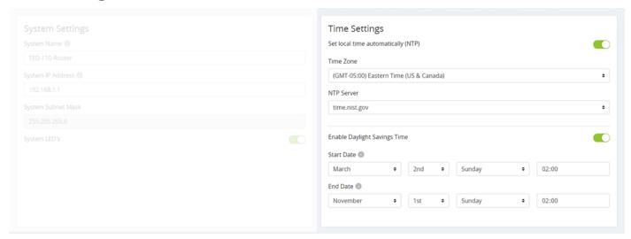
NTP: By default, the router checks the time automatically, using the NIST (National Institute of Standards and Technology) servers to synchronize to Coordinated Universal Time. This provides an accurate and
