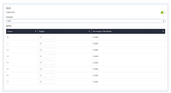
When WFQ is selected, you must assign the weight. Weight is a relative comparison of how important the data is. The router then adjusts the bandwidth assigned to each queue level according to these numbers.
