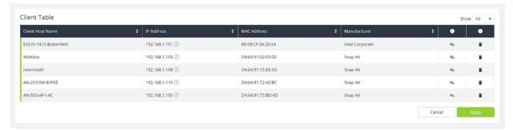
The client table section uses an ARP table to show all clients, their IP addresses (both DHCP and static), and their MAC addresses. The 310 models can support up to 500 client devices.
