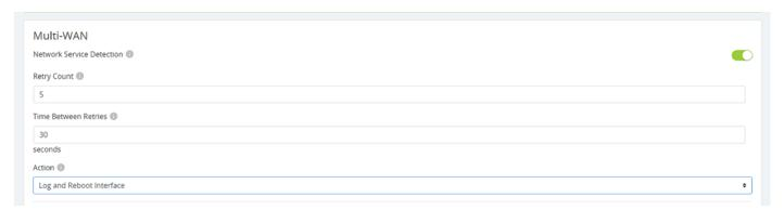
When Network Service Detection is enabled, you can opt to use any or all of the three detection methods listed to ensure your router is connected to the Internet. Actions are described below.
