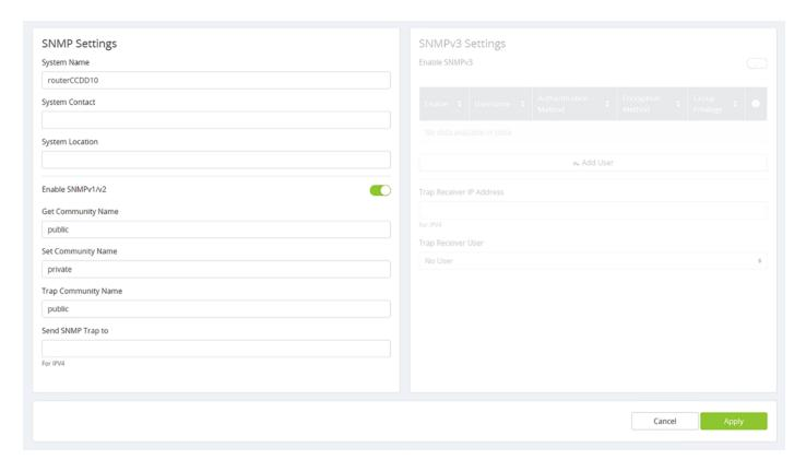
**System Name and Contact:** Use these to record the SNMP server manager's contact person and the server's physical location. Each of these parameters can be up to 64 characters. These identifiers are arbitrary and do not affect the server's function, but they are useful to have.
