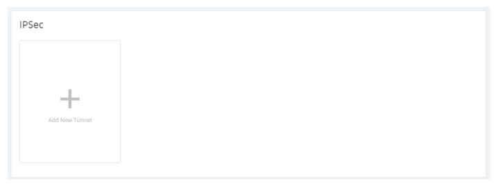
Click the + Add New Tunnel button to create a new IPSec tunnel.
